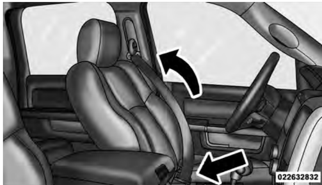
Removing Slack From Belt
